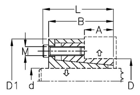
A mm = 37 B mm = 60.0 D1 mm = 96.5 d H8 mm = 40 D mm = 72 F kN torque = 105 L mm = 68.0 M mm = 8 P N/mm2 surface pressure on shaft/hub = 99
